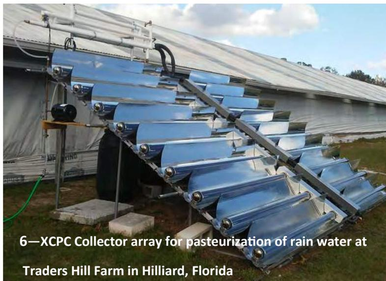
6—XCPC Collector array for pasteurization of rain water at Traders Hill Farm in Hilliard, Florida
