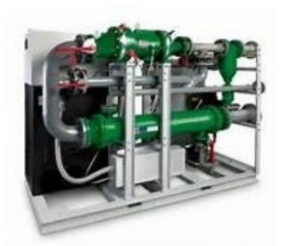
**ORC technology** transfers heat to a fluid with a low boiling point which is then vaporized, not unlike water powering a steam turbine. The ORC (organic Rankine cycle) engine allows power generation at lower capacities than the usual steam turbine or fossil-fueled generator. Combined with Artic Solar's XCPC it delivers low-cost, small scale, decentralized electricity generation.
